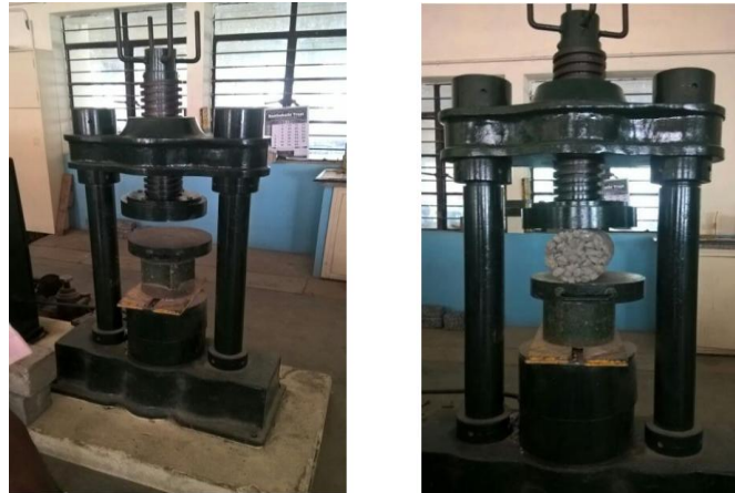
Fig-24 split tensile strength test
