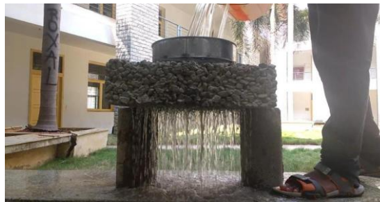
Fig-26 Permeability test
