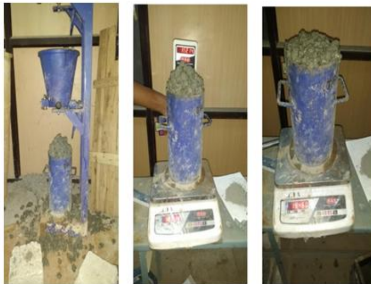
Fig-21 compaction factor test
